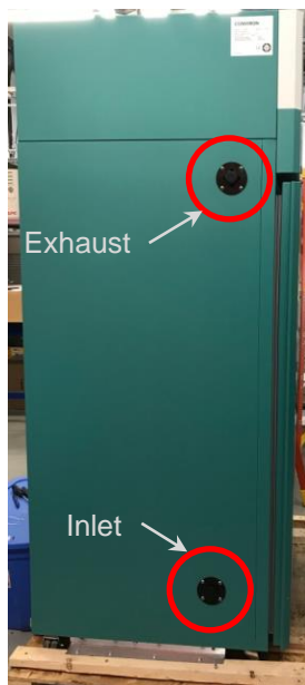
Figure 5-3 Fresh Air Inlet and Exhaust Port Location
