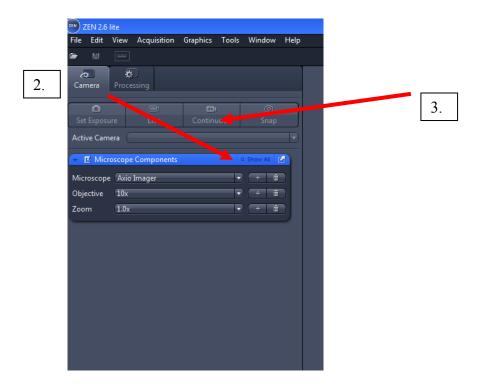
2. For example, click on the Mirosccope Components Tab. Confirm that correct light path (i.e., objective, filters, etc.). For example if usng the 20x objective select that option. If usng the FITC channel filter, select for that option.
